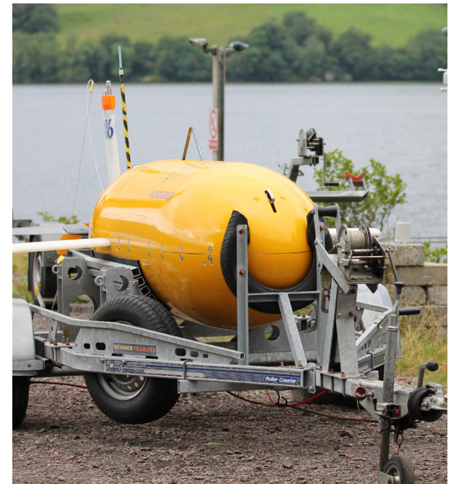
Autosub Long Range being prepared for under-ice capability testing in Loch Ness
