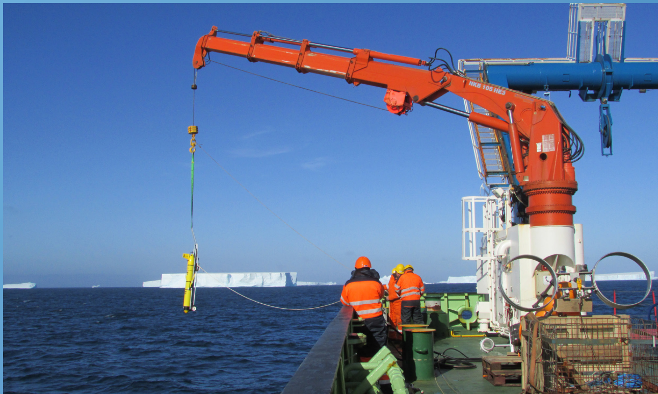
Glider being deployed using the new in water release trolley for the first time
