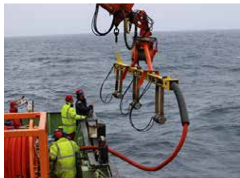
◀ Image preparing to deploy the seismic source
