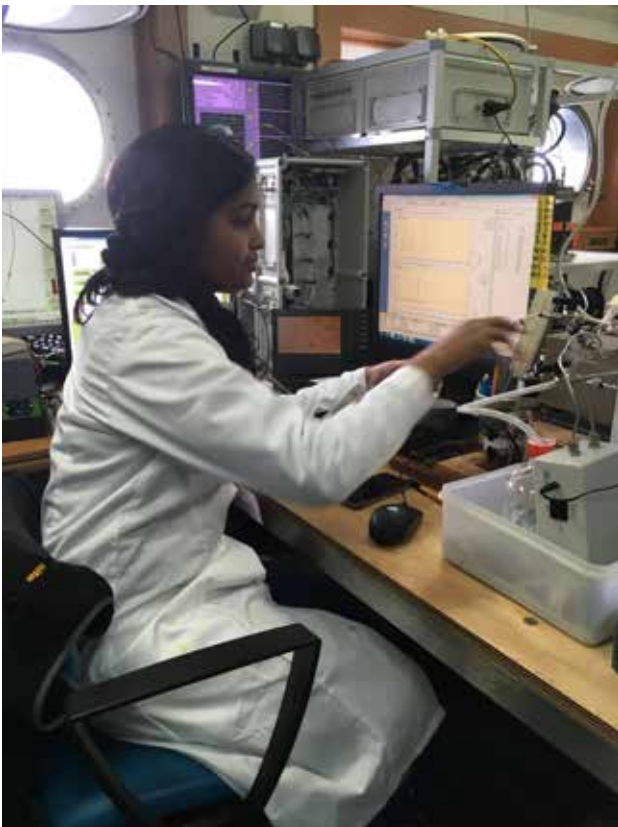
▲ Christabel Fernandes an AMT-POGO sponsored fellow from Goa, India measuring dissolved nitrous oxide and methane on CTD collected seawater
