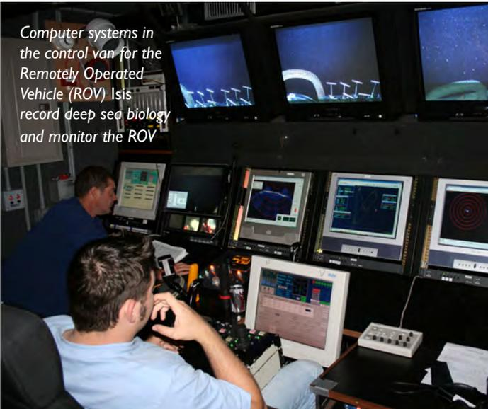
Computer systems in the control van for the Remotely Operated Vehicle (ROV) Isis record deep sea biology and monitor the ROV
