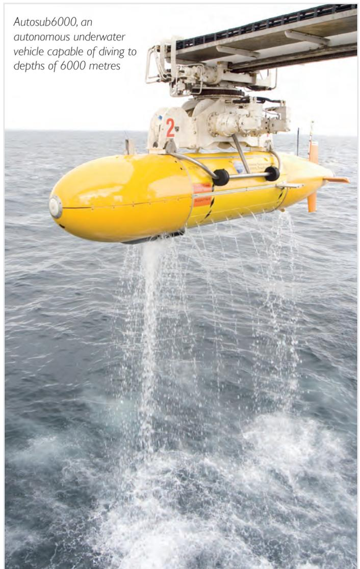
*Autosub6000, an autonomous underwater vehicle capable of diving to depths of 6000 metres*
