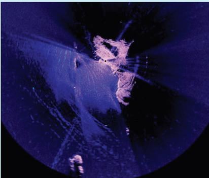
State of the art NOC marine radar remote sensing of coastal seas was demonstrated at a proposed Tidal Energy development site through a project with Meygen Ltd. Some of the capabilities of this technology include bathymetric survey, current measurement, sea surface roughness and small target tracking (marine wildlife, both airborne and seaborne).
