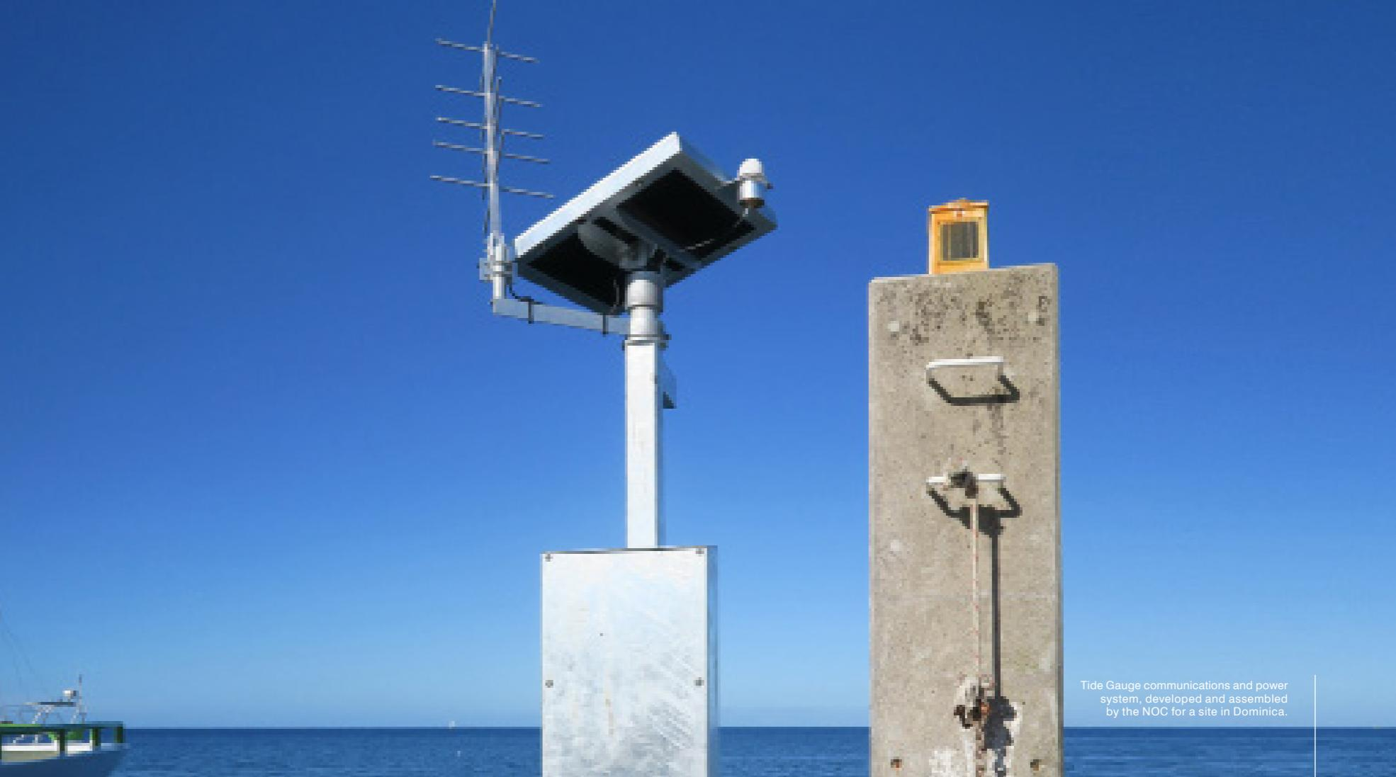
Tide Gauge communications and power system, developed and assembled by the NOC for a site in Dominica.
