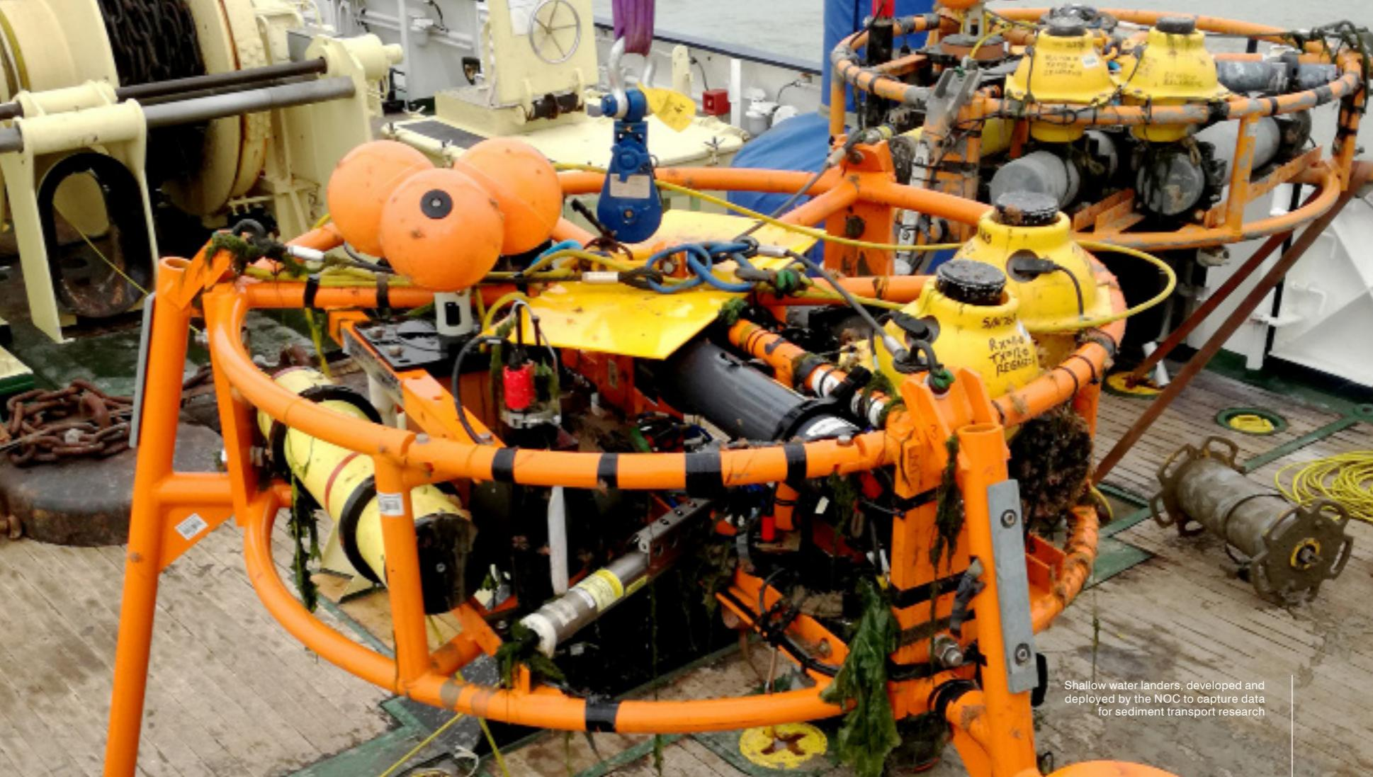
Shallow water landers, developed and deployed by the NOC to capture data for sediment transport research
