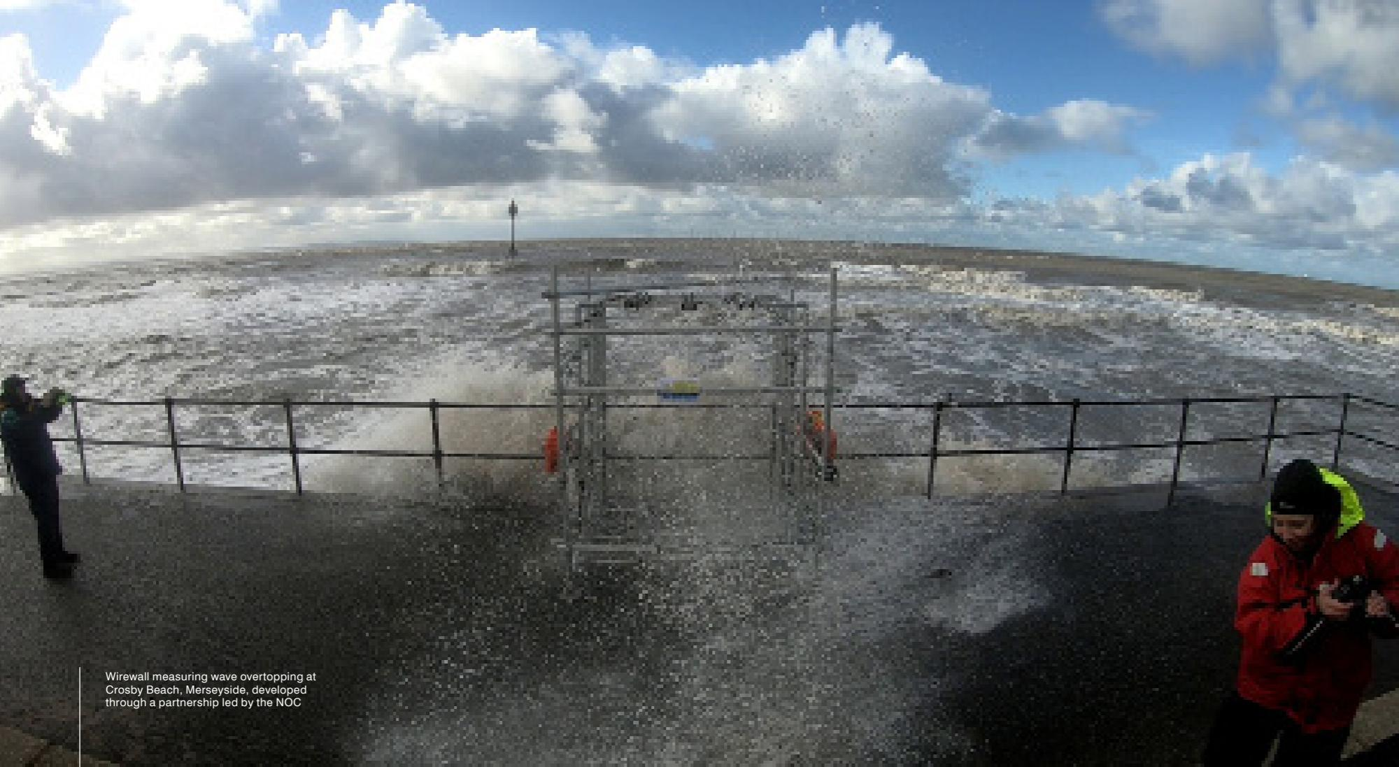
Wirewall measuring wave overtopping at Crosby Beach, Merseyside, developed through a partnership led by the NOC
