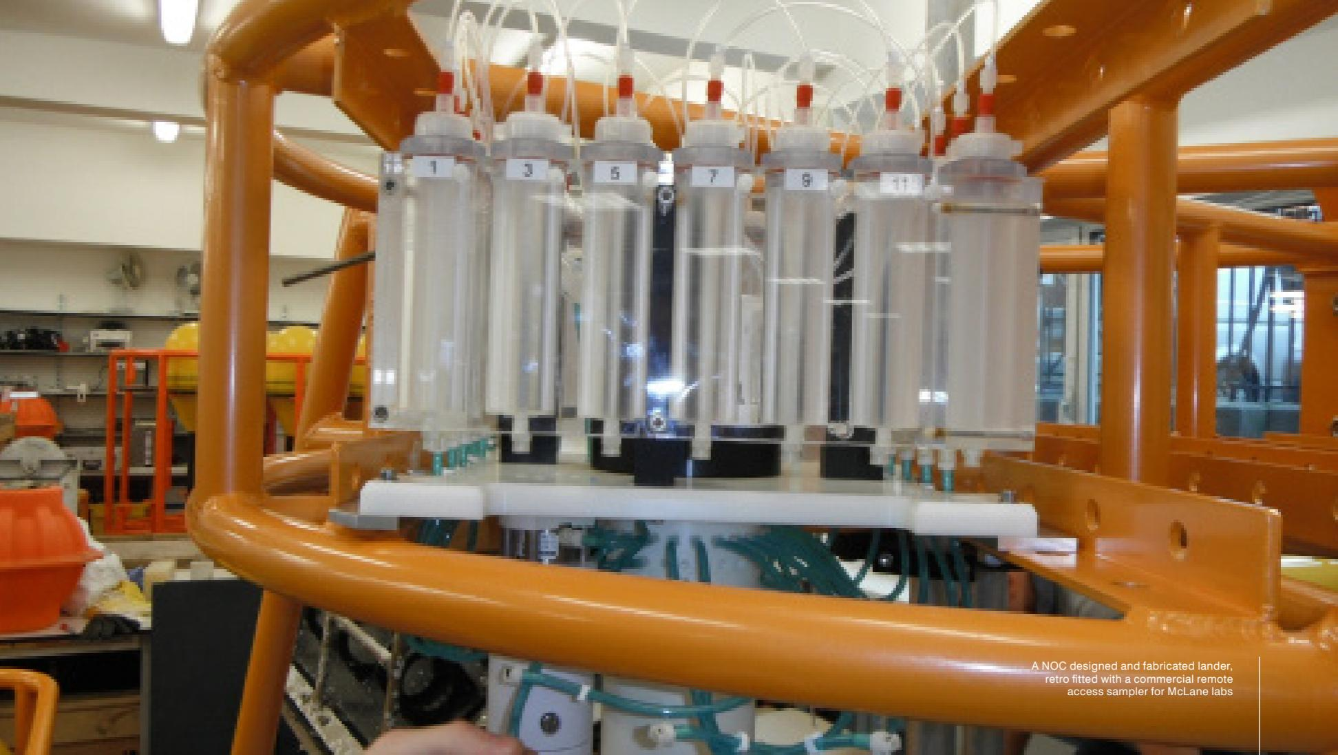
A NOC designed and fabricated lander, retro fitted with a commercial remote access sampler for McLane labs
